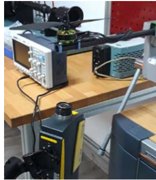
Fig. 9. Polytec PDV 100 laser vibrometer placed under the electric motor
