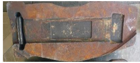
Fig. 4 Visual testing and measurement of worn zones for reconditioning a) Worn part that needs reconditioning; b) Part that does not require reconditioning
