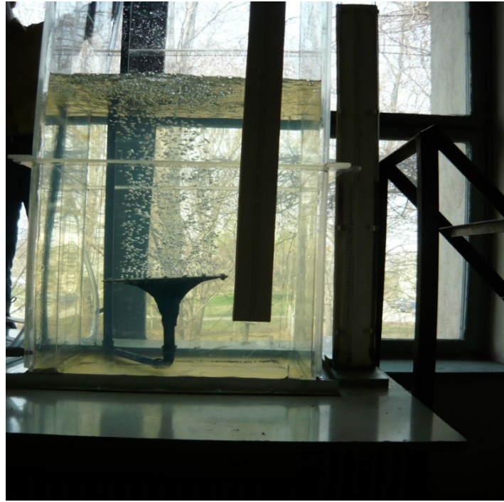
Fig.6. FBG in function; \Delta h_1 = 60 \text{ mbar} = 611 \text{ mmH}_2\text{O} .
