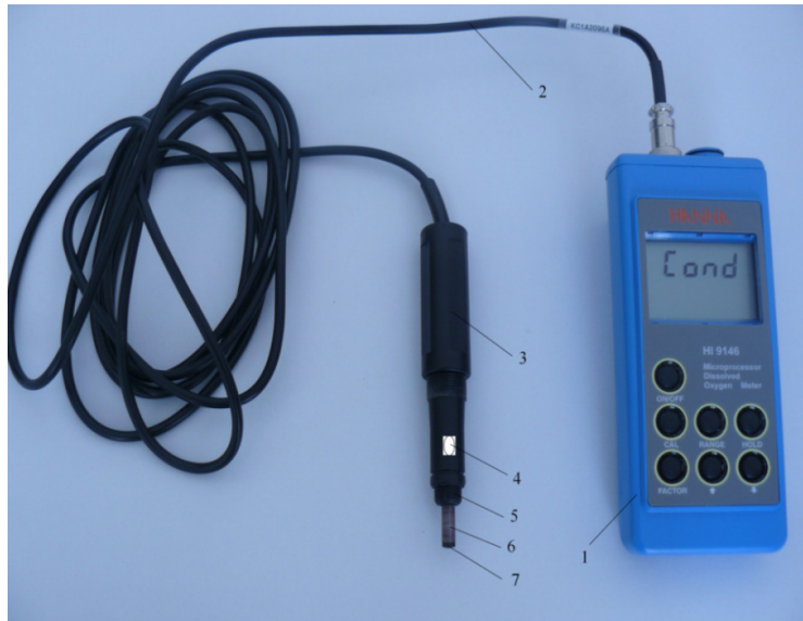
Fig. 1. General view of the oxygen meter: 1- microprocessor with digital display; 2 – connection cable; 3 – probe body; 4 – temperature sensor; 5 – threaded portion of the probe body where the part 4 (fig.2) is screwed; 6 – anode; 7 – cathode.
