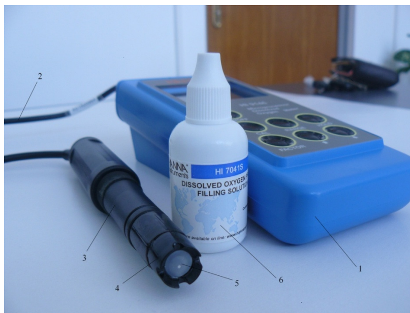
Fig. 2. Assembly view of the oxygen meter prepared for measurements. 1- microprocessor; 2 – connection cable; 3 – probe body; 4 – small cylinder that contains an electrolyte solution; 5 – oxygen permeable Teflon membrane; 6 – solution vial.
