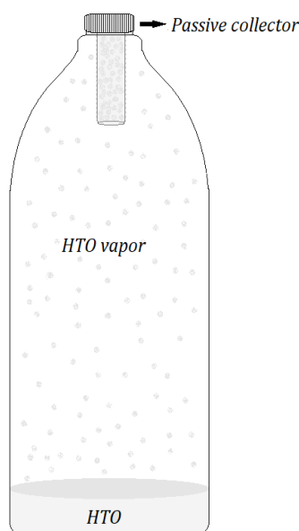
Fig. 3. The experimental arrangement for determining the accuracy of the method
