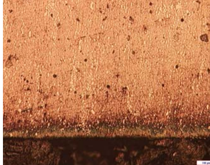
Fig. 4. The microstructure of the ion nitrided layer and of neighbored zone. Rp3 (HS18-0-1) steel, after advanced plastic deformation, heat treatment (quenched and triple tempered) and ion nitriding (450°C/1.5h; \delta \sim 150\mu\text{m} ) Nital 5%
