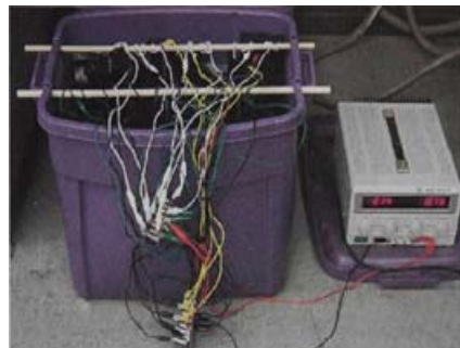
Fig.2 - Galvanic Corrosion Cell -Front View
