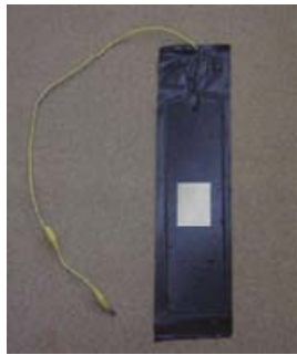
Fig.1 - Masked Specimen Showing Exposed Area to Be Corroded
