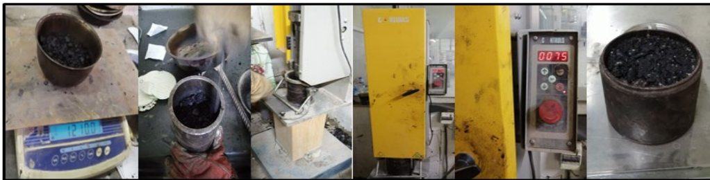
Fig. 7. Marshall mould, Marshall hammer and number strikes.
