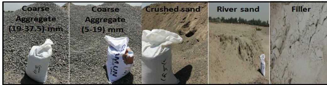
Fig. 4. The materials used in the asphalt mixture (base layer).
