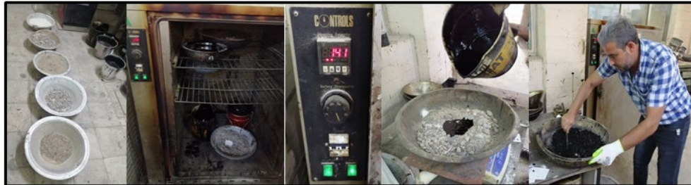
Fig. 5. Asphalt mixture materials in the furnace and mix them manually.
