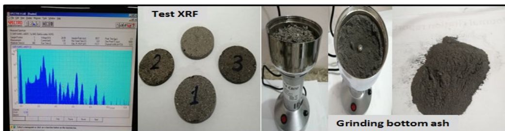
Fig. 3. XRF test for bottom ash and its grinding
