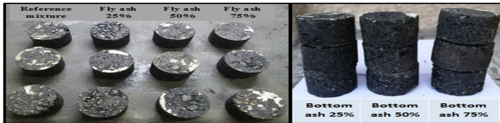
Fig. 6. Marshall Specimen with the addition of fly ash and bottom ash.
