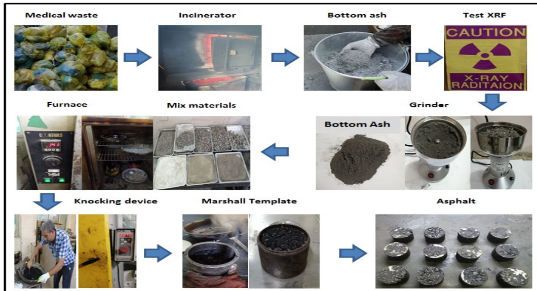
Fig. 1. The stages of converting medical waste into bottom ash and mixing it with the asphalt mixture.
