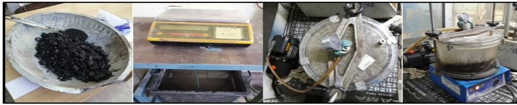
Fig 9. Theoretical specific gravity device
