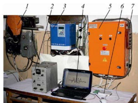
Fig. 4. Control and data acquisition station of the experimental bench based on the electric hoist with a capacity of 0.5 t
