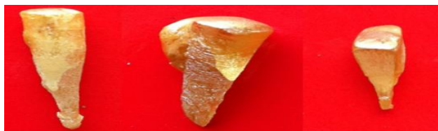
Fig. 1. Sample of rutile single crystal with growth failure
