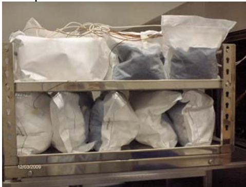
Fig 5. Position of transducers inside the autoclave
