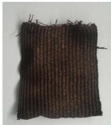
Fig. 11 Composite textile with inserted microwires for electromagnetic shielding
