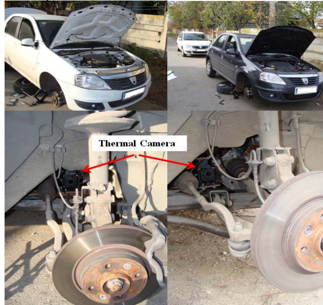
Fig. 3. Position of thermal camera on test motor vehicles Left – unvented brake disc; right – vented brake disc
