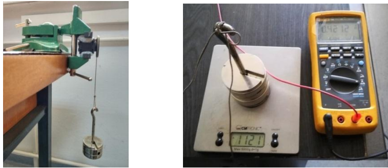
Fig.7. Set up for determination of the servo characteristic
