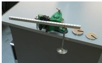
Fig.2. Set up for measuring static friction
