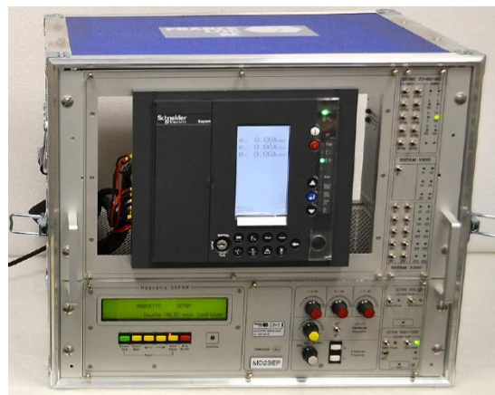
Fig. 11. The MD2ADSEP pedagogical platform with the S80 numerical overcurrent protective relay introduced
