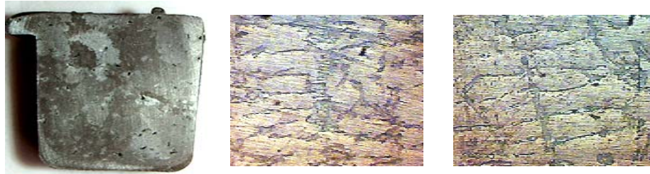
3 inside the pyramid : a. macrostructure (1:1); b. microstructure of the edges (x100); c. microstructure in centre.
