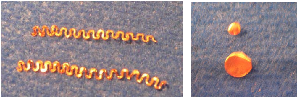
Fig. 1. The electrodes: left - the ground electrode, right - the active electrodes
