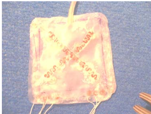
Fig. 3. The ground electrodes fixed on the envelope
