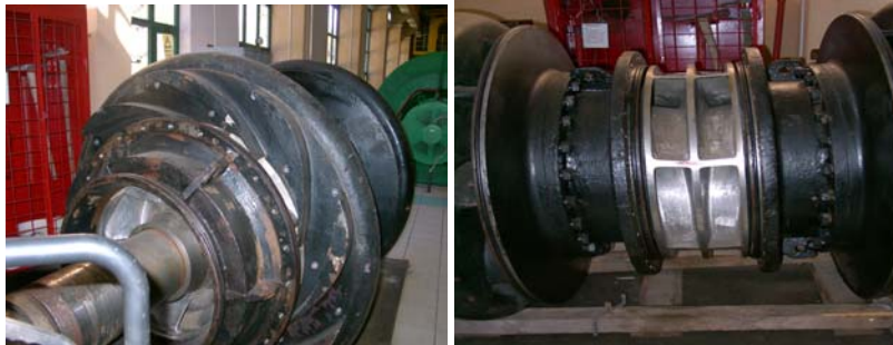
Fig. 1. Double stage and double flux storage pump
