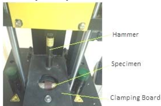
Fig. 4 . The impact hammer and the clamping method for impact
