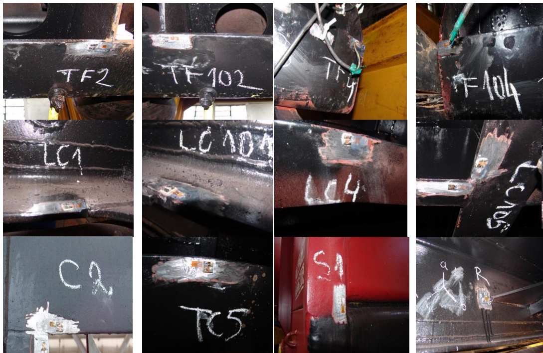
Fig. 6. Strain gauges mounted on the vehicle structure
