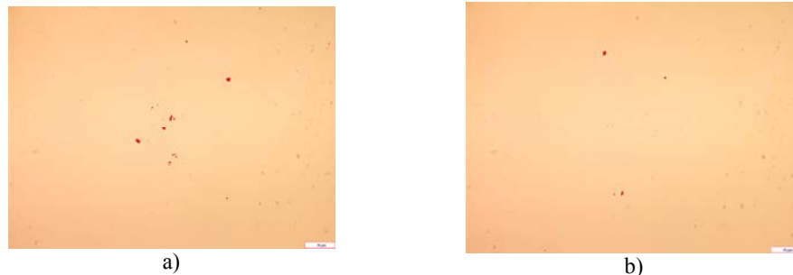
Fig. 2.2.1 Captured and processed image for pin E1 on a)longitudinal and b) transverse cross-section
