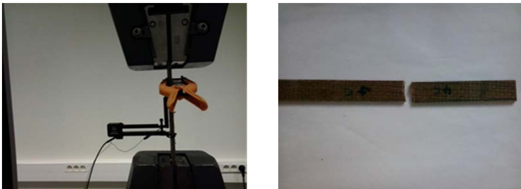
Fig. 1. Tensile static test for eco-composite specimen
