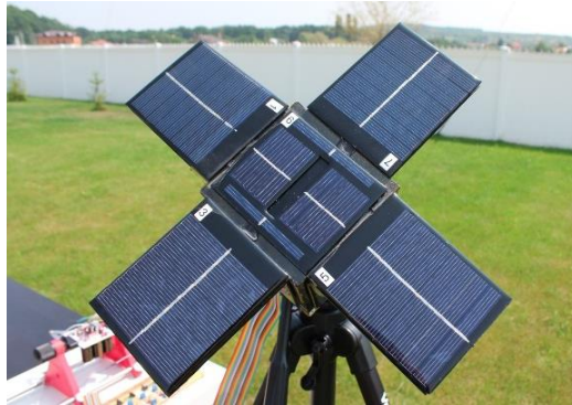
Fig.7. The physical model of the testing nanosatellite with the solar panels extended towards sun.
