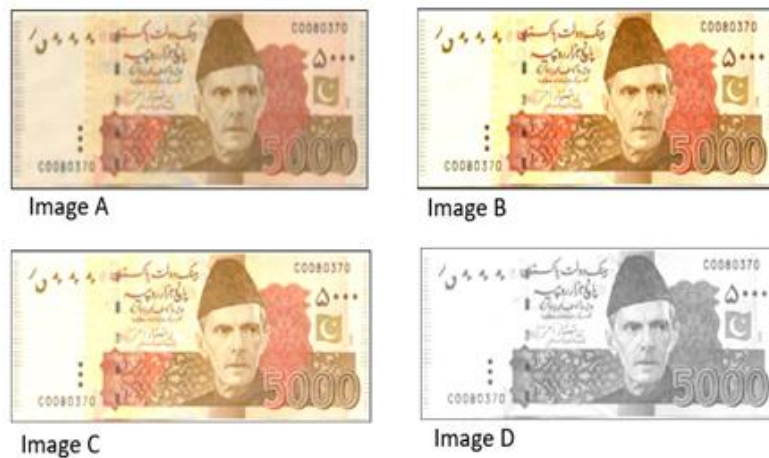
Fig. 2. The image of Pakistani currency when processed with different pre-processing techniques: smoothened currency note, brightened currency note, blurry currency note, and gray-scaled currency note.
