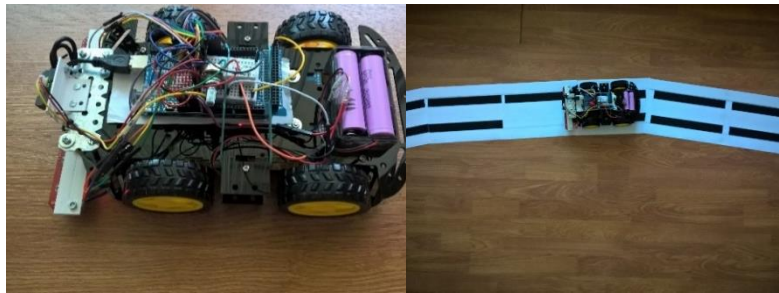
Fig. 4. Test car based on Arduino (left), contains sensors for detecting track markers, radio communications module for interacting with the system, and a compass for determining movement bearing. On the right, example of track markers.
