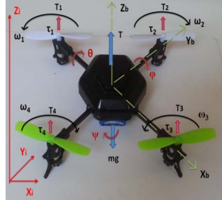
Fig. 2. Conceptual model of a quadrotor dynamics
