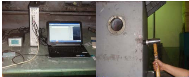
Fig. 11. LMS Test.Lab10B modal analysis system & Impact hammer
