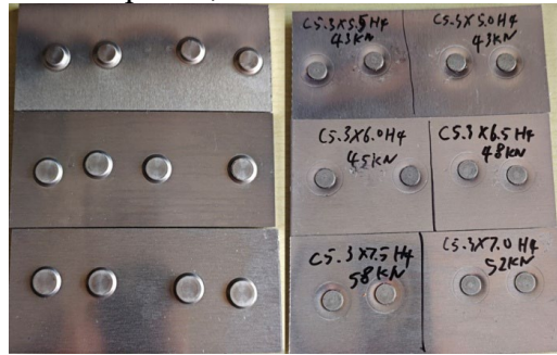
Fig. 7. Test specimens for double-rivet connection
