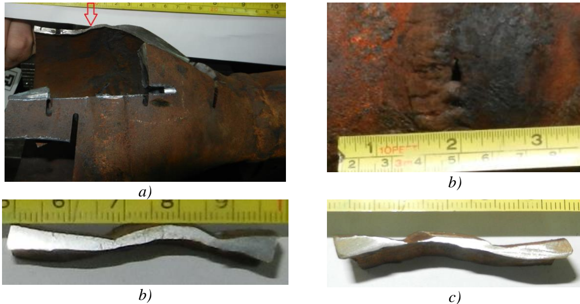
Fig. 6. The macroscopic aspect of the eccentric reducer DN50 / DN100 welded joint with the pipe elbow DN100 in the porosity zone. a) joint overview after sectioning; b) detail of the joint surface in the porosity zone; c) section in the pipe wall at 30 mm distance from the porosity; d) section in the pipe wall where the porosity is located.
