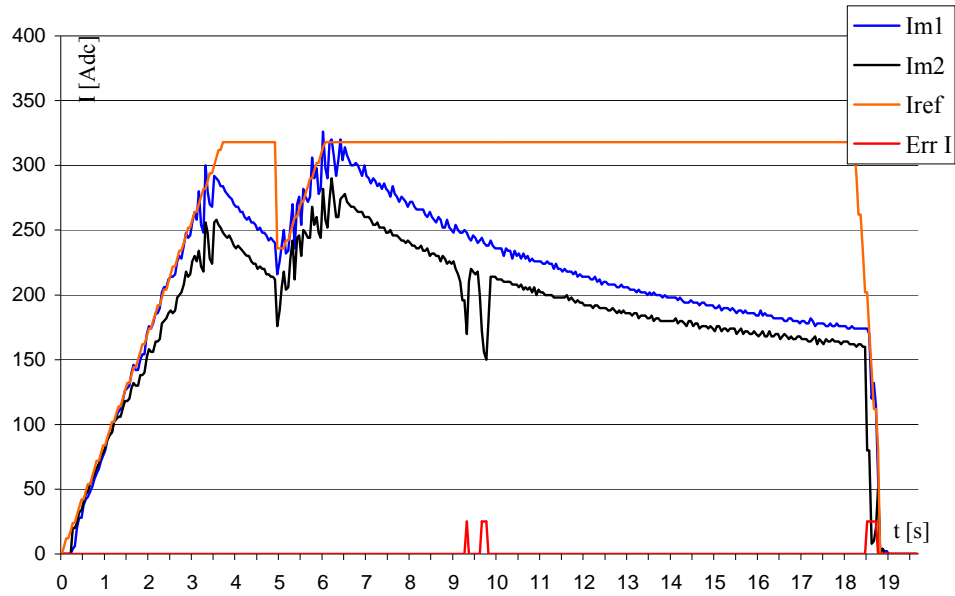
Fig. 9 The experimental diagrams of the current reference ( I_{ref} ), motor currents ( I_{m1} and I_{m2} ) and vehicle's speed ( V ) during the slip protection tests
