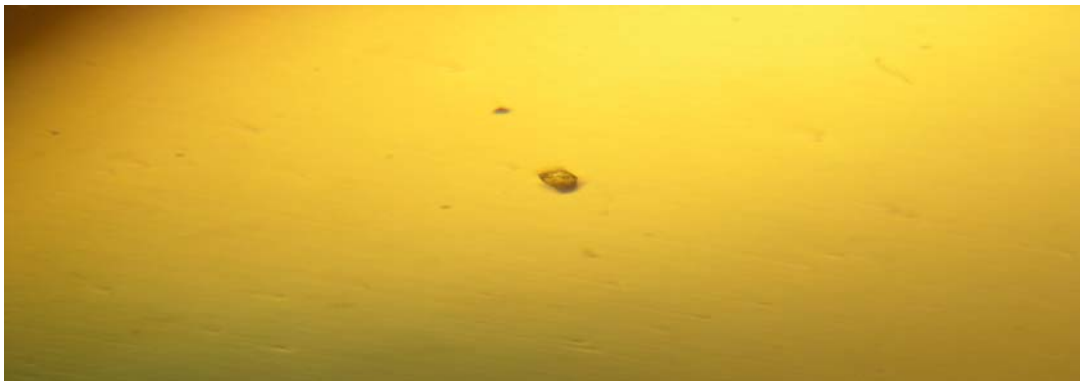
Fig.4. Image with metallographic microscopy for sample 1 magnification of 100\times (globular inclusions)
