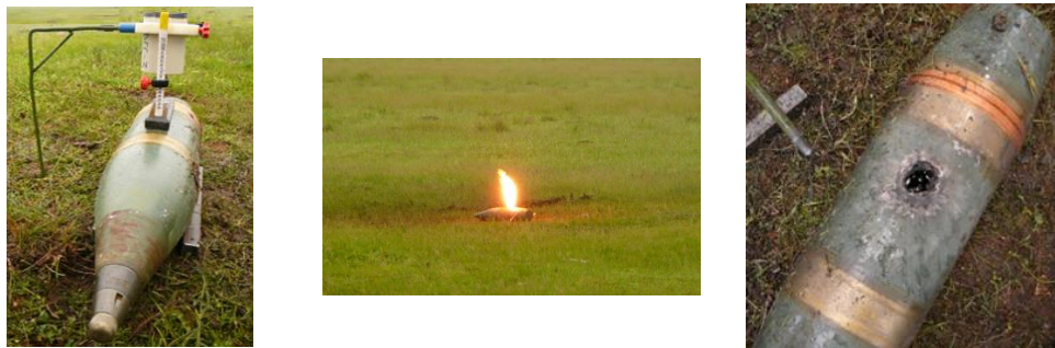
Fig. 3. Stages of UXO neutralization
