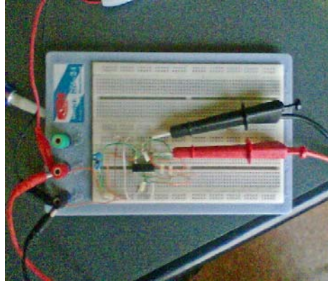
Fig. 4. Experimental set-up, the neural controller on a quick board.
