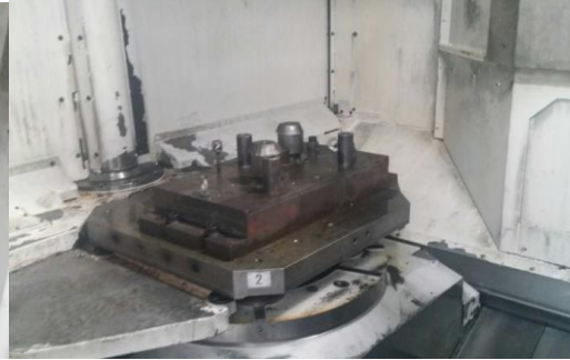
Fig. 7. The workpiece fixture structure
