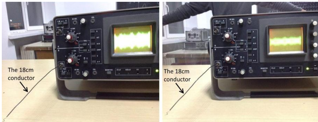
Fig. 1. Perturbing signal caught in the didactic laboratory on a 18cm long conductor, connected to the input of a 150MHz band oscilloscope, on the 0.1 V/div. and 50 ns/div. scale. One can see the initial signal (left side), and the one reduced by 6dB (right), during a simple directive shielding test scenario
