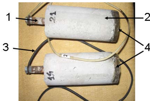
Fig. 1. Reinforced concrete samples made by mixing cement, standard sand and water: 1 – steel rebar; 2 – concrete; 3 – copper wire; 4 - epoxy resin insulation.
