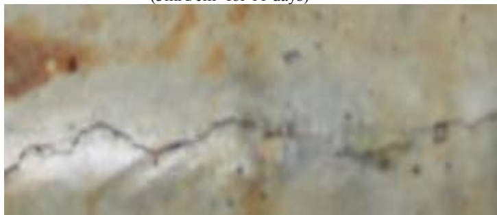
Fig. 5. The appearance of reinforced concrete sample exposed to cathodic polarization ( 3\text{mA}/\text{cm}^2 for 11 days)
