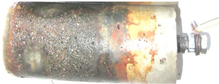
Fig. 4. The appearance of reinforced concrete sample exposed to a.c. polarization ( 3\text{mA}/\text{cm}^2 for 11 days)
