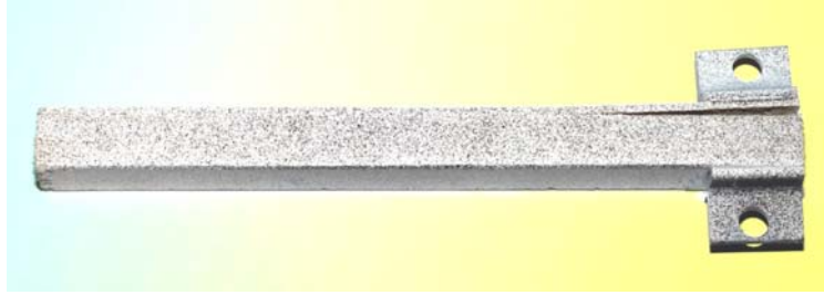
Fig. 6. Sandwich composite specimen prepared for testing.
