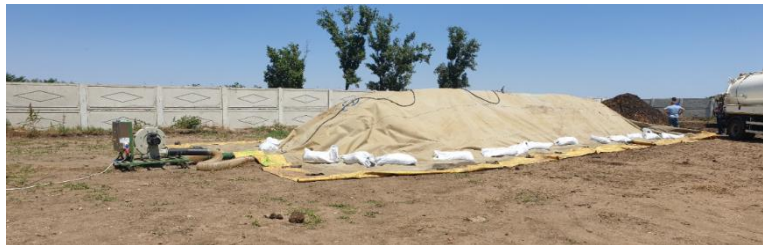
Fig. 4. Semi-permeable membrane and automatically controlled forced aeration system (original - Inoveco)
