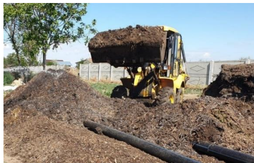
Fig. 10. Turning the stack after the first 28 days (original - Inoveco)
