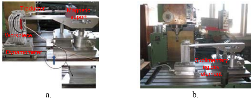
Fig. 21. Clamping device during tests: a.- Rising the device from the machine table, b. - Assembly with supplementary stiffening elements
