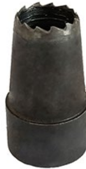
Fig.2 Carbide annular serrated blade used in the test
