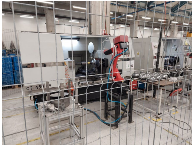
Figure 2 – Robotic arm working on CNC machine in Glorious Lighting
