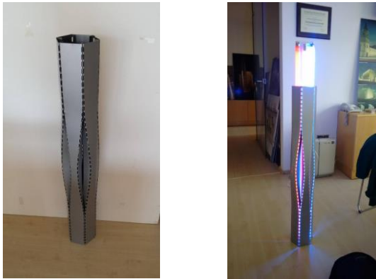
Fig. 19. Metallic prototype (stamping with elongated perforations)
