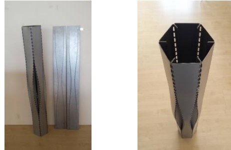
Fig. 18. The metallic experimental model (stamping with elongated perforations)
