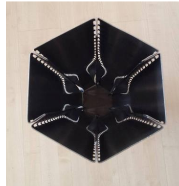
Fig. 20. The metallic experimental model (stamping with elongated perforations)
