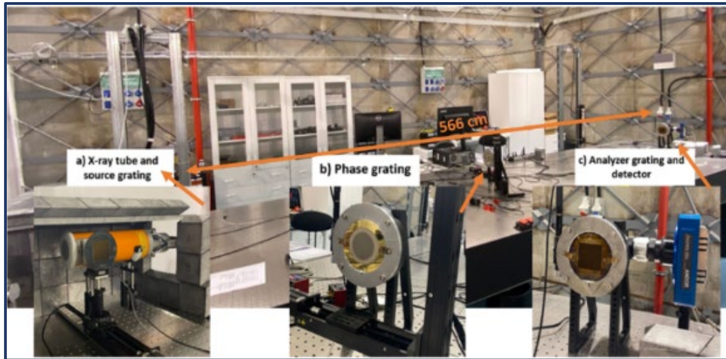
Fig. 6. Photo of Talbot-Lau Interferometer from the X-ray Imaging Laboratory from ELI-NP.
