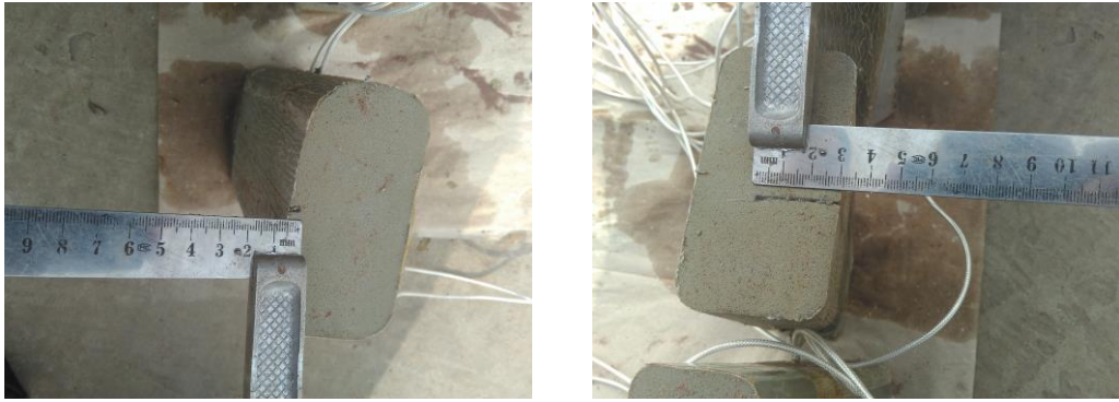
Fig. 2. Measurement of the maximum cutting depth
