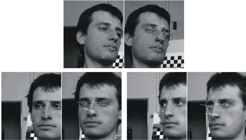
Fig. 6: Results of head orientation and position estimation as well as gaze vector estimation.
