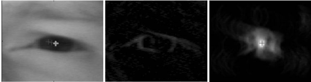
Fig. 4: Iris center detection: the eye patch with the detected iris center, the edge map and the Hough likelihood map
