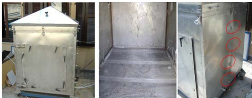
Fig. 2. Pilot plant, internal view and details regarding the probe temperature position
