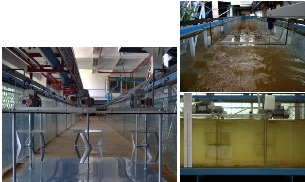
Fig. 1. Experimental set-up: Hydropower farm model at 1:5 scale (left frame); Variable slope open channel (upper-right frame); Turbine models turning in water (lower-right frame)
