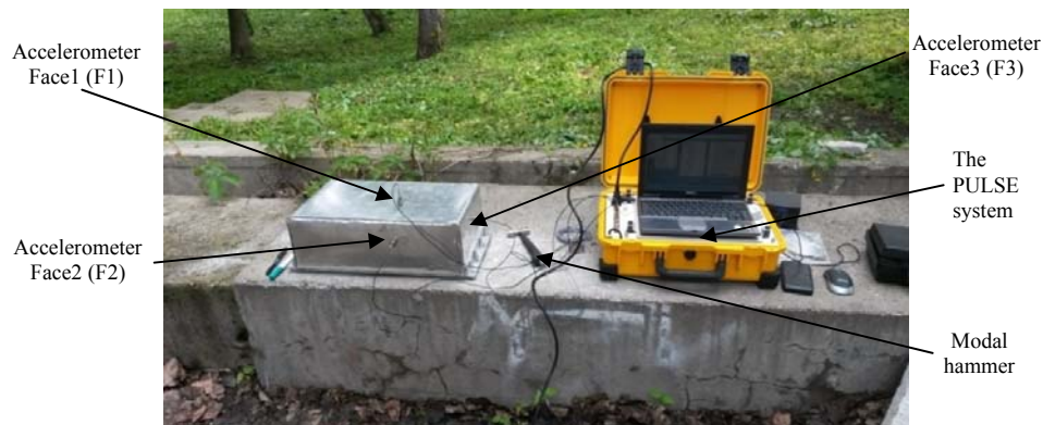
Fig. 2 Experimental set-up for natural frequencies measurement
