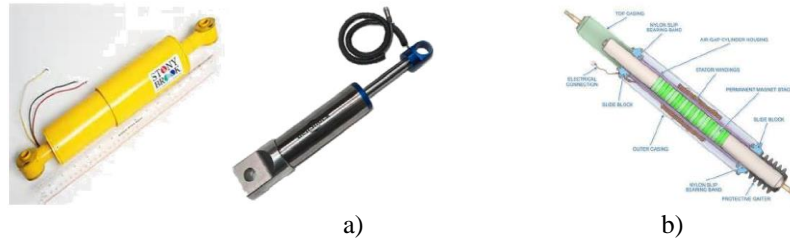
Fig. 1. PGSA Suspension Energy Recovery System, [2] a) presentation of the system; b) system detail
