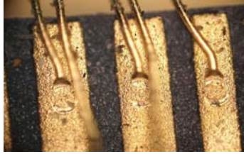
Fig. 2 Micro-joining types of "wedge bonding" the golden wires
