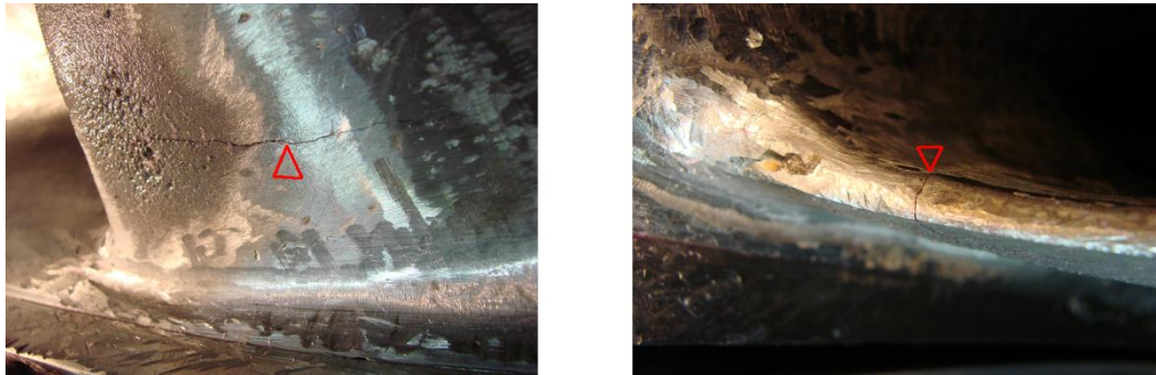
Fig. 6. Cracked runner blade at the band limit (left). Trailing edge crack at the blade/band limit (right)
